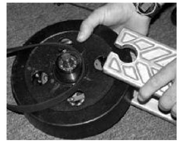
Step 5. Remove Bracket to Check Belt
