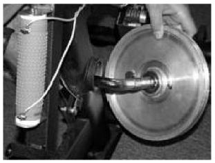
**Step 5.** Remove Large Pulley Assembly.
