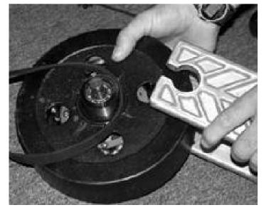
Step 5. Remove Bracket to Check Belt
