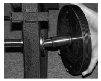
Step 2. Slide Shaft Through Frame
