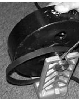
Step 2. Pry Bearing Out of Housing
