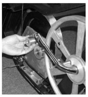
**Step 1.** Remove Small Poly-V Pulley
