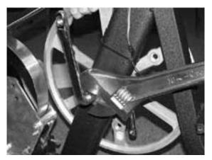
Step 1. Remove Crank Nut.
