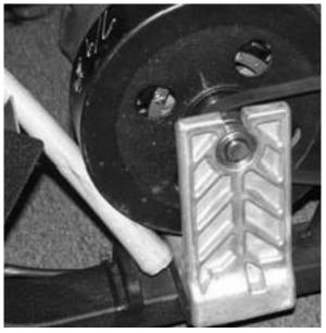
Step 3. Pry on Brake to Loosen Belt.
