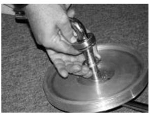
Step 8. Remove Bearing & Washer
