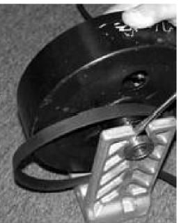
Step 2. Pry Bearing Out of Housing
