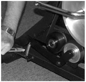
Step 1. Belt Tensioning Spring
