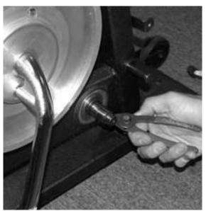
Step 1. Remove Shaft Snap Ring on Right Side
