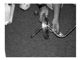
Step 9. Pull Crank Thru Pulley to Remove
