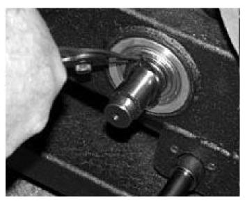
Step 1. Remove Snap Ring on Right Side
