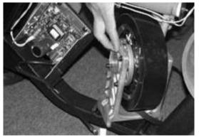
Step 7. Remove Brake & Belt Assembly
