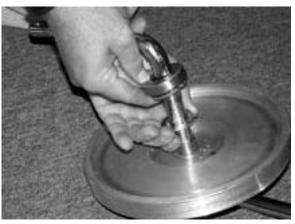
Step 8. Remove Bearing & Washer
