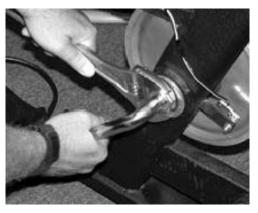
Step 1. Remove Crank Nut.
