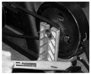
**Step 3.** Pry on Brake to Loosen Belt.
