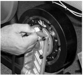
Step 5. Disconnect Wiring Harness.
