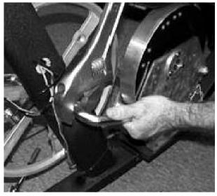
Step 1. Remove Crank Nut
