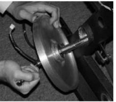
Step 5. Remove Large Pulley Assembly.
