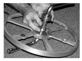
Step 8. Remove Bearing & Washer
