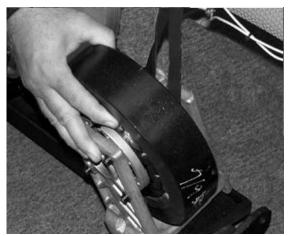
Step 7. Remove Brake & Belt Assembly
