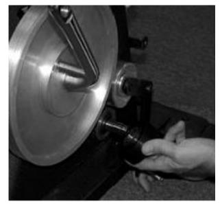
**Step 2.** Remove Small Poly-V Pulley
