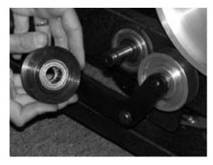
**Step 5.** Remove the small poly-V pulley
