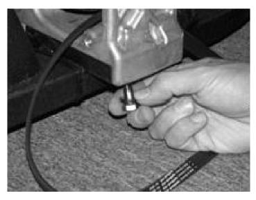
Step 2. Loosen Bracket Bolts
