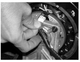
**Step 5.** Disconnect Wiring Harness.
