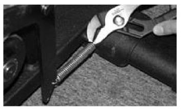
Step 1. Remove Belt Tensioning Spring
