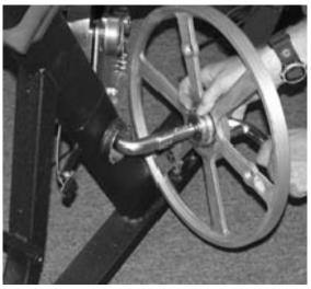
**Step 5.** Twist Unit Thru Hub Frame. Copyright 2001 True Fitness Technology, Inc.
