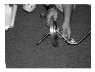
Step 9. Pull Crank Thru Pulley to Remove
