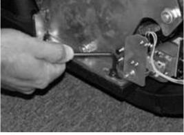
Step 4. Loosen Hub Bracket Screws
